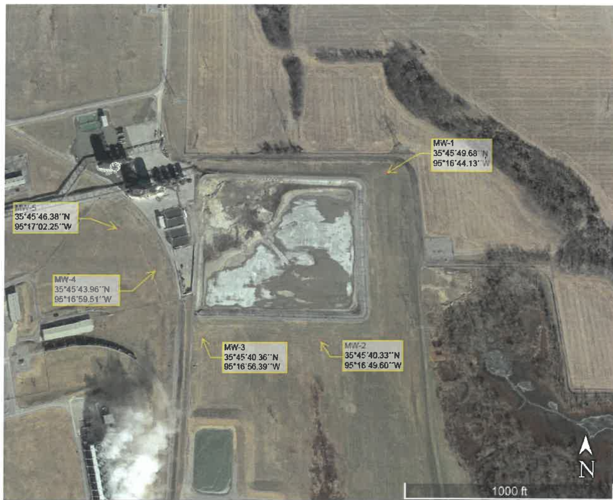
Figure 2-1 Monitoring Well Location Map
